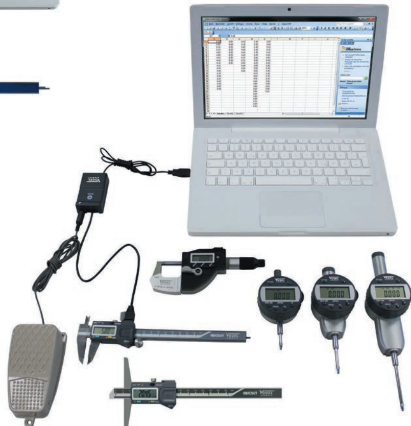
2. example data processing via Duo-Data output (for our USB interfaces or for Mitutoyo Digimatic)
