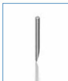
Stylus tip 13 mm Order no.: 101-030-130 made of carbide, \varnothing 1 mm / R: 25 \mu m / A: 19°
