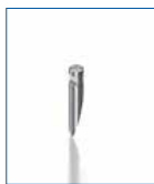
Stylus tip 20.5 mm Order no.: 101-010-205 made of carbide, \varnothing 3.5 mm / R: 25 \mu m / A: 12°
